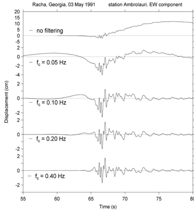
Figure 13. Displacement time-histories for a series of filters with different parameters.
