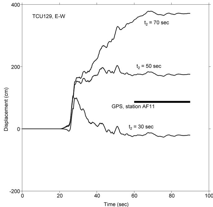
**Figure 22.** Displacements obtained by double integration of the east-west component of acceleration recorded at TCU129 from the 1999 Chi-Chi, Taiwan, earthquake and modified using a variety of baseline corrections. The GPS level was obtained at a station 2.3 km from TCU129, above the footwall of the fault (as is TCU129). (From [41]).
