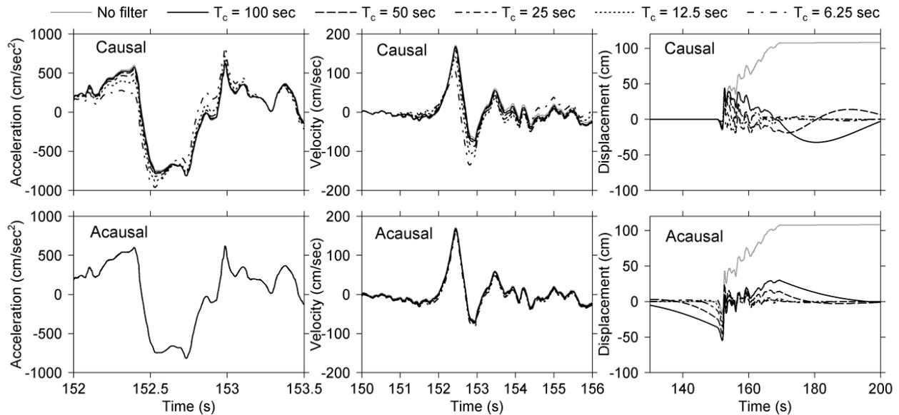
**Figure 10.** Accelerations, velocities, and displacements from the 228 degree component of the analog recording at Rinaldi during the 1994 Northridge earthquake for causal (*top*) and acausal (*bottom*) filtering. The time scales are different for the acceleration, velocity, and displacement time series to better display certain features.
