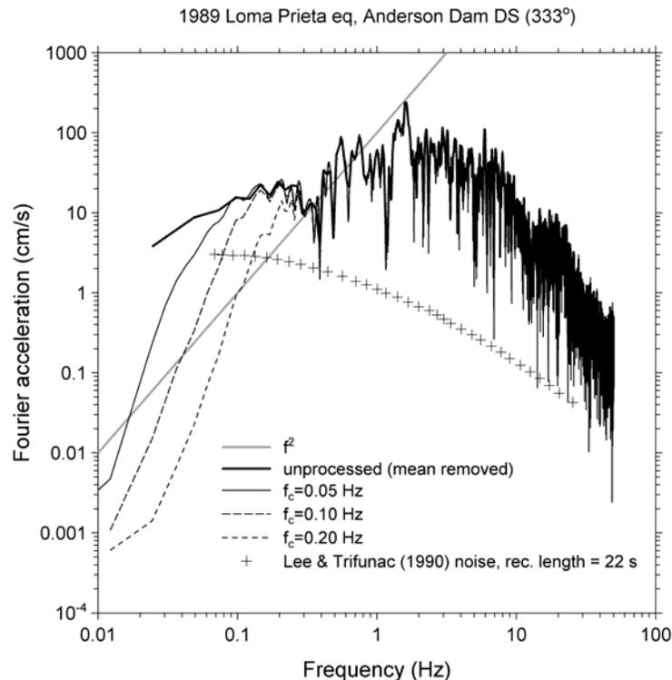
**Figure 17. Fourier acceleration spectrum of a digitized version of an analog recording for three values of  $f_c$ . Also shown is the theoretical low-frequency slope for a single-corner source model, and representative noise curves from Lee and Trifunac [6], from which a signal-to-noise ratio of 3 would suggest that the filter corner should be near 0.06 Hz.**
