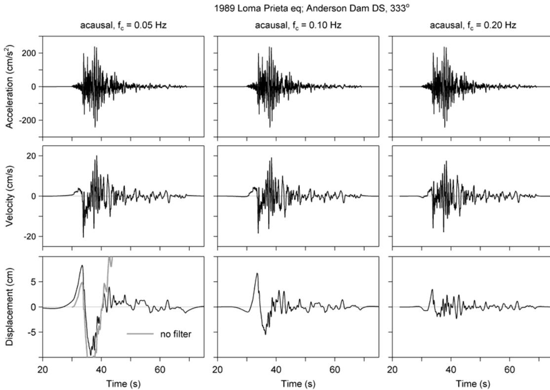
**Figure 18.** Acceleration, velocity, and displacement using three values of  $f_c$ . The displacement from the unfiltered acceleration is shown in gray.
