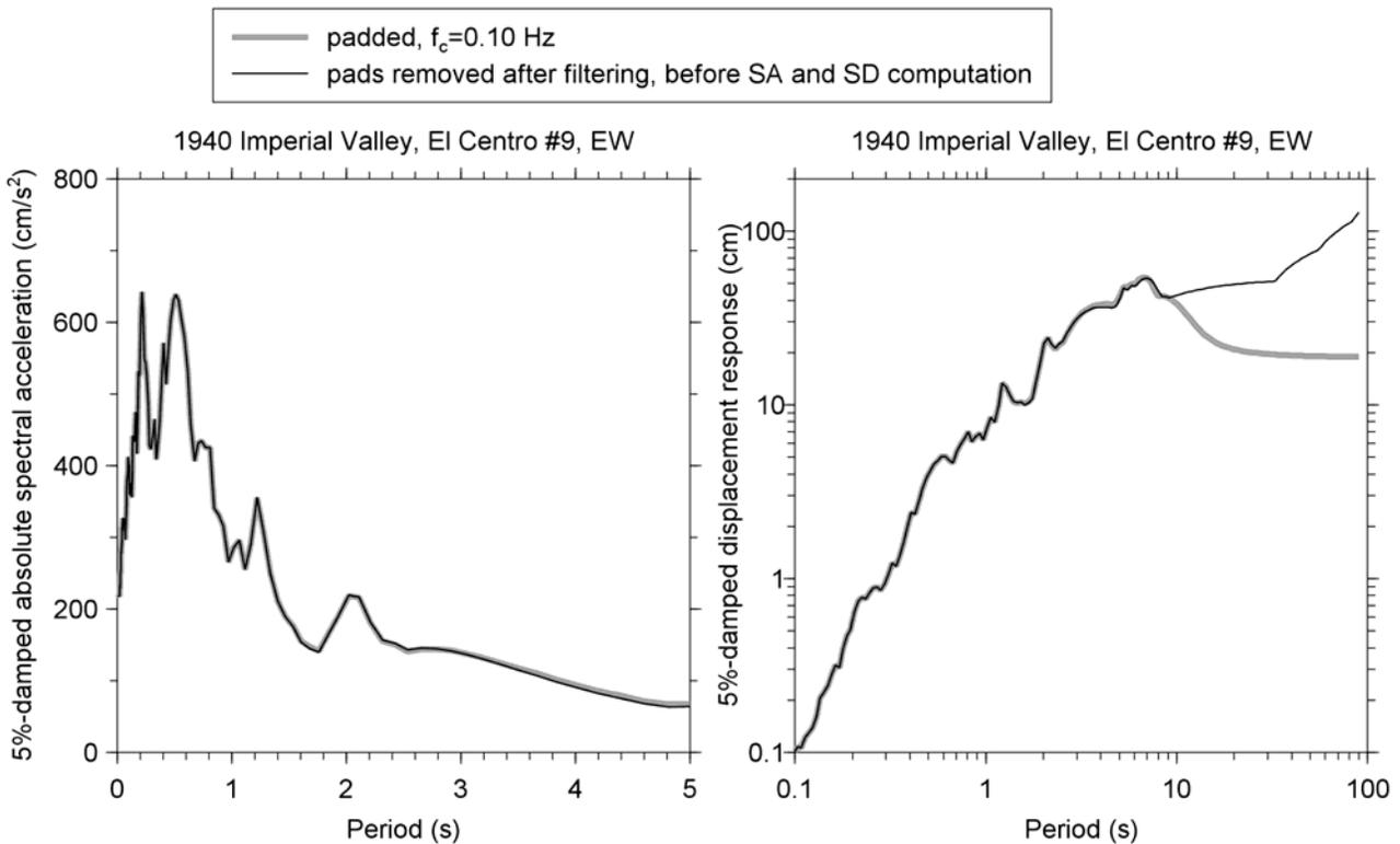
**Figure 2.** Absolute acceleration response (SA) and spectral displacement (SD) computed for the El Centro station 9 recording of the 1940 Imperial Valley earthquake, from the filtered acceleration before and after removal of the zero padded portion. Note that SA and SD have been plotted using linear and logarithmic axes, respectively.
