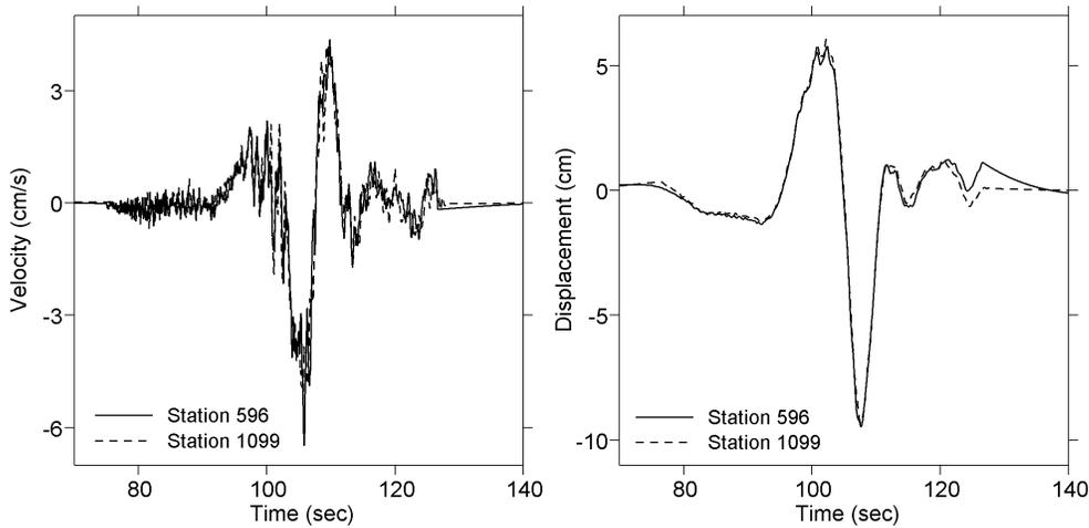
**Figure 21.** Comparison of the processed velocity and displacement traces from the N-S components of two stations located about 1.6 km apart and about 160 km west of the  $M_w$  7.2 Hector Mine earthquake in 1999. Note the remarkable similarity between the signals at these two stations, particularly at long periods. Comparisons such as this are used to confirm that proper filter corners were selected to process the records.
