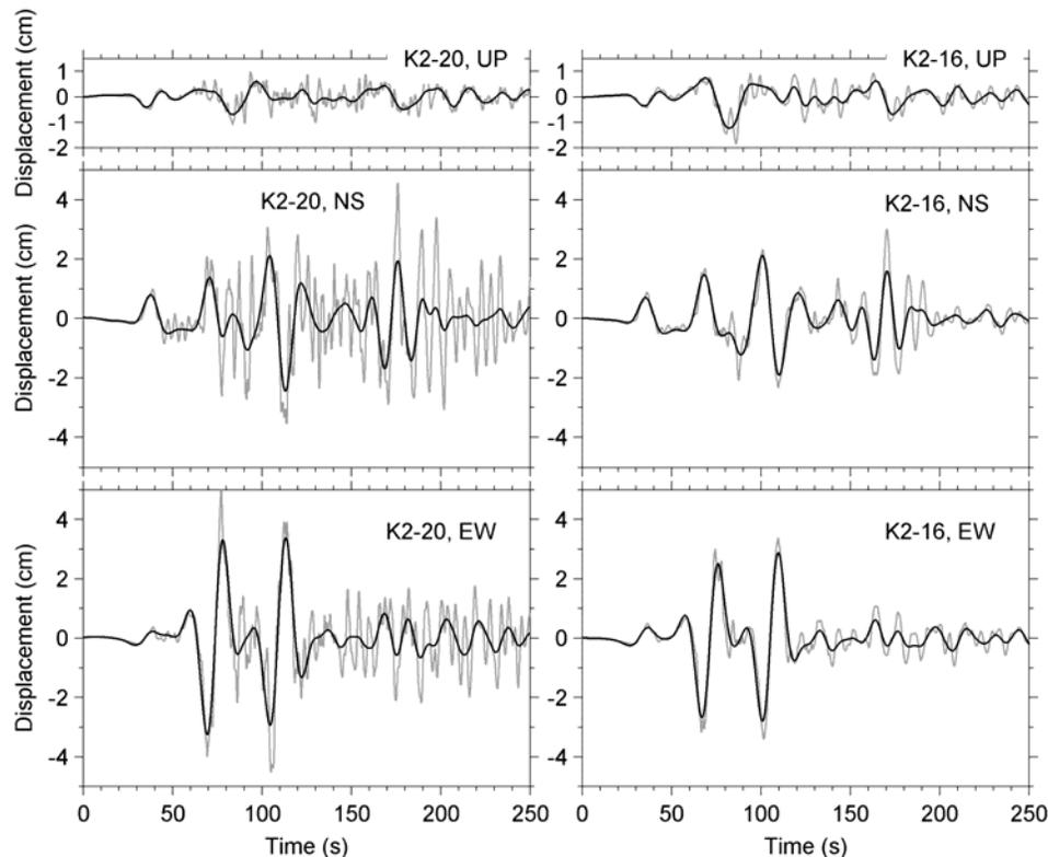
**Figure 20. Displacements at stations K2-16 and K2-20 (see Figure 19), showing the strong coherence at low frequencies. Station K2-20 is on lower velocity materials and has more high frequency motion than does station K2-16. Gray curves have been low-cut filtered at 0.02 Hz; black curves have been low-cut filtered at 0.02 Hz and high-cut filtered at 0.08 Hz.**
