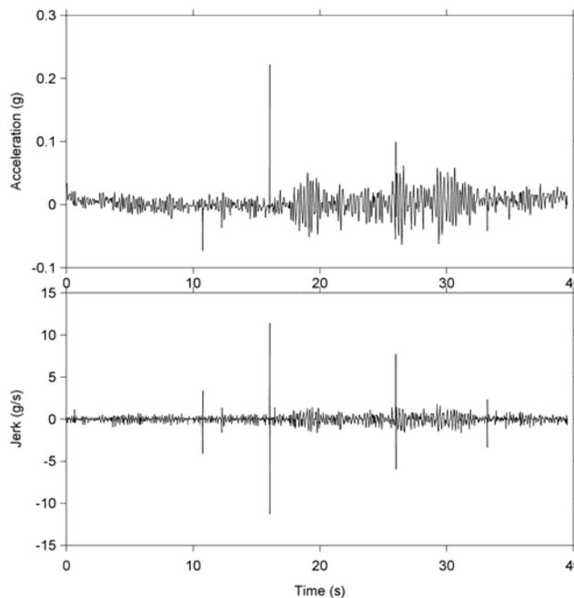
**Figure 3.** Horizontal component of the Bajestan recordings of the 1978 Tabas earthquake in Iran; spurious spikes are obvious in the acceleration record at 10.8 and 16 sec. The derivative of the acceleration trace (to produce the quantity called “jerk”) will convert a spike into a double sided pulse, making it easier to identify spikes. By doing this (bottom panel), spikes at 12.3, 26 and 33.2 sec are also identified.
