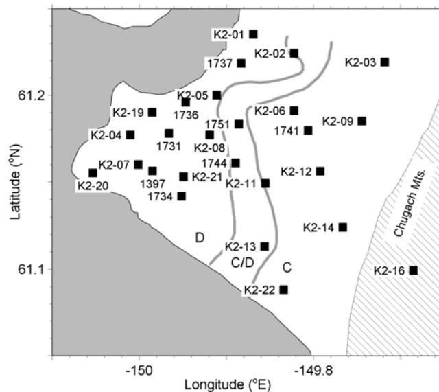
**Figure 19.** Location of stations and NEHRP site classes (site classes and base map from Figure 12 in [39]). The C/D class is intermediate between NEHRP classes C and D, and is defined here by the average 30 m shear wave velocity being between 320 and 410 m/s [39].
