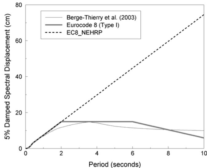
**Figure 7. Displacement response spectra for rock sites due to a magnitude 7 earthquake at a hypocentral distance of 15 km obtained from the equations of Berge-Thierry et al. [14] and from Eurocode 8 [15]. The dashed line shows the form of the EC8 spectrum if the same corner.**
