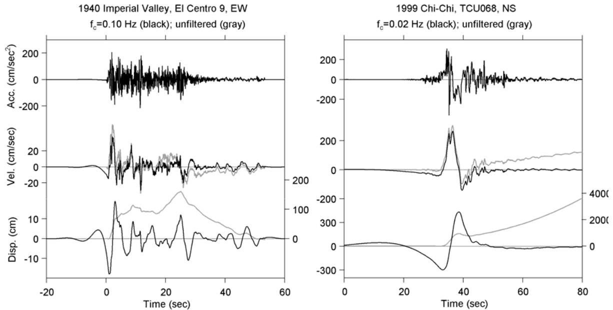
**Figure 12.** Acceleration, velocity and displacement from the analog and digital recordings; the only processing for the gray traces was to remove the overall mean for the analog record and the prevent mean for the digital record. The black traces show the velocities and displacements derived from acceleration time series filtered as indicated. The displacement axis labels for the unfiltered motions (gray) are given on the right side of the graphs.
