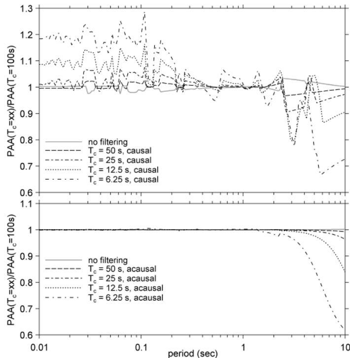
**Figure 11.** Ratio of 5%-damped pseudo absolute acceleration spectra (in  $\text{cm/s}^2$ ) from the 228 degree component of the analog recording at Rinaldi during the 1994 Northridge earthquake for causal (*top*) and acausal (*bottom*) filtering, using the results for a filter corner of 100 sec as reference.
