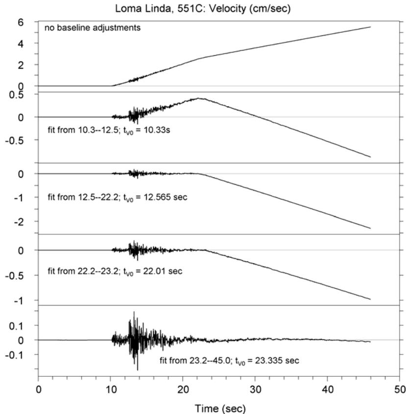
**Figure 16. Sequential baseline adjustments applied to the velocity time-history obtained from integration of a digital accelerogram with shifts in the baseline. Note the change in the ordinate scales of the plots.**
