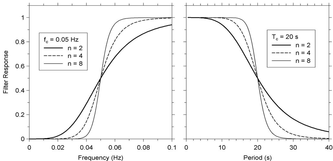
**Figure 8.** Illustration of a low-cut Butterworth filter as a function of frequency and period. The filter frequency is 0.05 Hz, which means that periods above 20 sec are at least partially removed. The different curves are for different orders of filter: the higher the order, the more abrupt the cut-off. For the lower order filters, information will be removed from periods as low as 10 sec.
