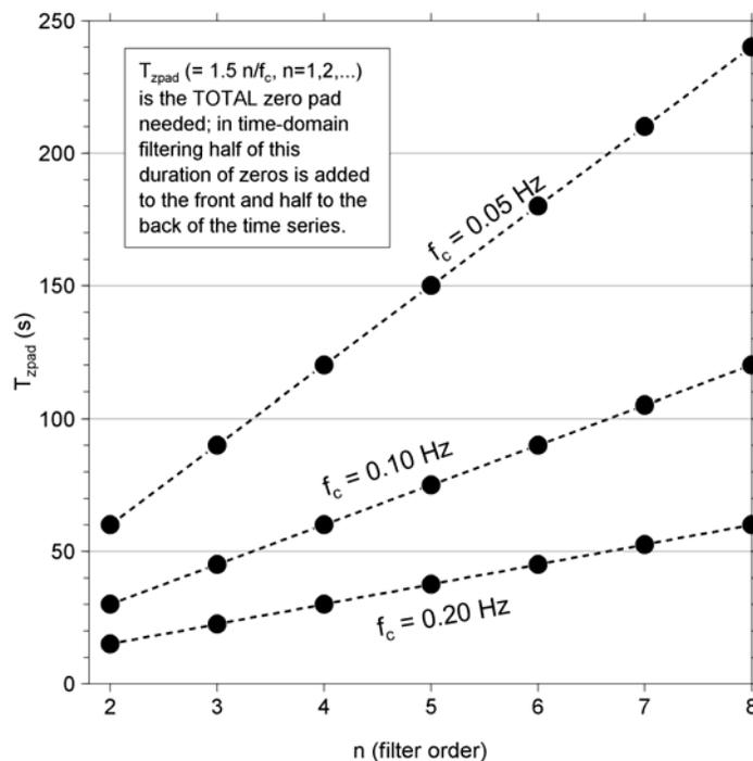
**Figure 9.** The total length of the time-domain zero pad recommended by Converse and Brady [7] to allow for the filter response in 2-pass (acausal),  $n^{\text{th}}$ -order Butterworth filters (these pads are needed regardless of whether the filtering is done in the time- or frequency-domain). Pre- or post-event data count as part of the required pad length. Shown are the pad lengths for three values of the filter corner frequency, as a function of filter order.
