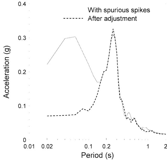
Figure 4. Acceleration response spectra (5% damped) from the accelerogram in Figure 2 before and after removal of the spikes.
